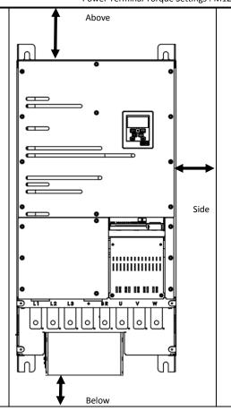
Required Mounting Clearances for Cabinet Installation
